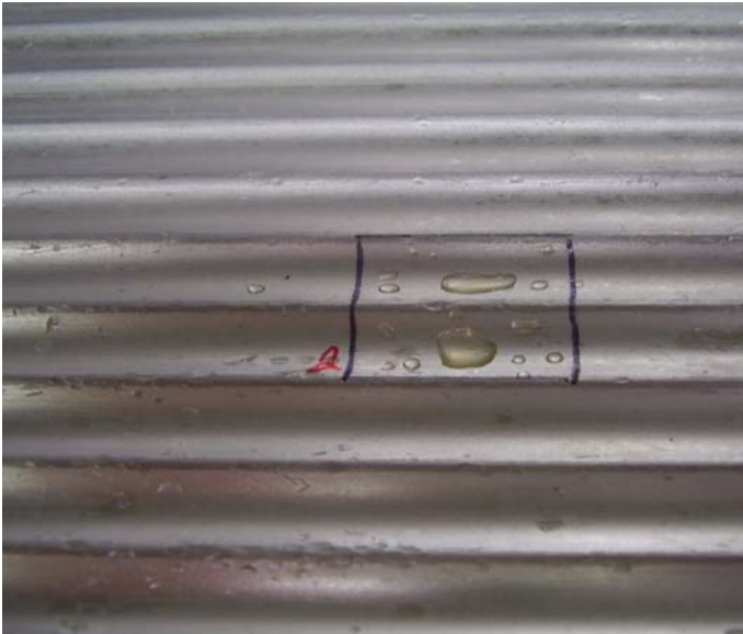
Figure 1: Cast aluminum component with marked gridded area after inoculation of 40 ul L. innocua .
